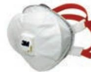
**3M™ Particulate Cup Shaped Respirator 8825+ and 8835+ Series** have been engineered to help improve fit to wearer's individual face shape and size. With a robust shell and cup design, these respirators meet the particular requirements of the clogging test for FFP (filtering face piece) respirators and is EN 149 'R' rated which means that they may be used for more than one shift.
